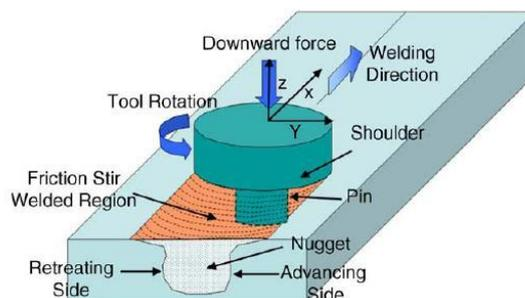
Fig. 1. Schematic drawing of friction stir welding.
