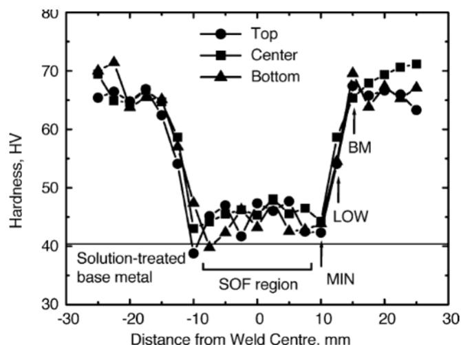
Fig 4. Typical hardness curve across the weld of FSW 6063Al-T5 [20]
