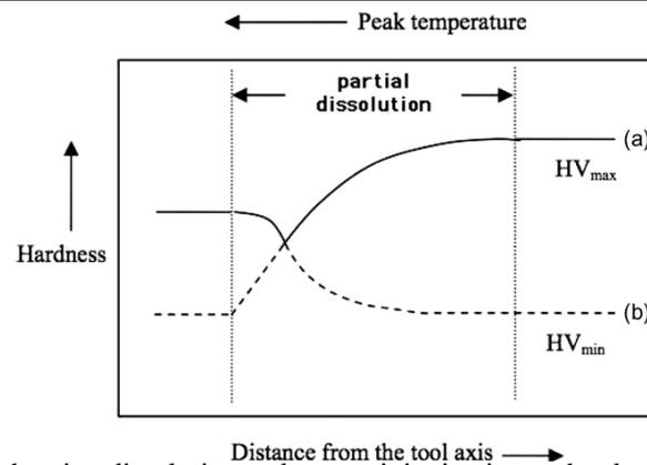
Fig. 3. A schematic diagram showing dissolution and re-precipitation in age-hardenable aluminium alloys. HV denotes the Vickers hardness number. Adapted from [25].
