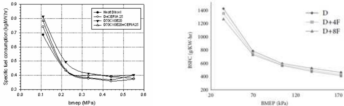
Figure-2 Variation of BSFC with BMEP with respect to engine load at 2200 rpm
