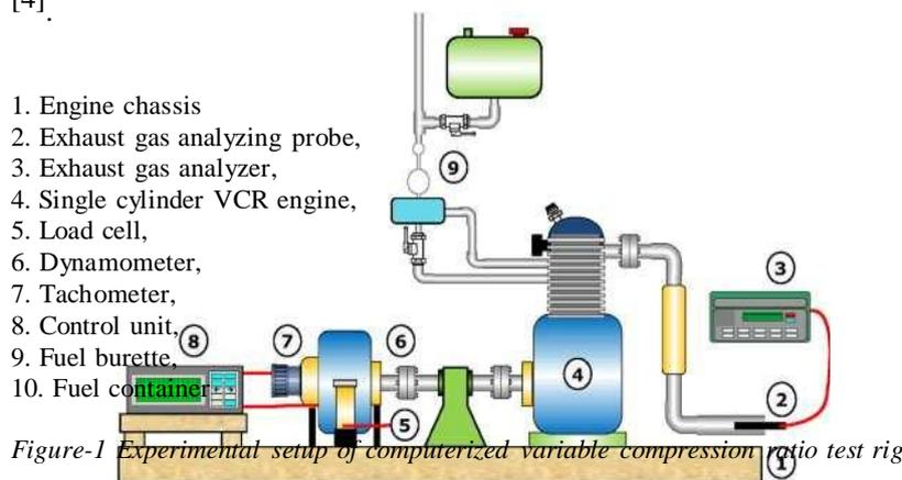
Figure-1 Experimental setup of computerized variable compression ratio test rig
