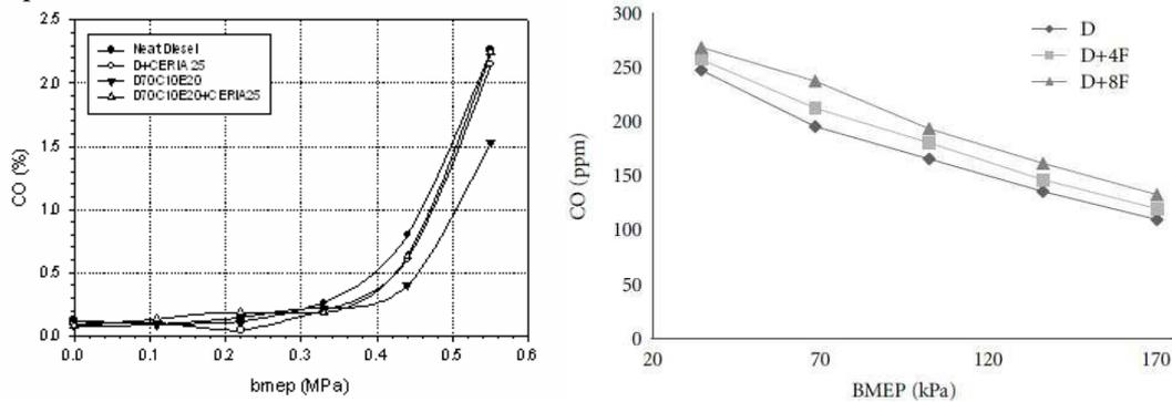
Figure-4 Variation of CO with BMEP with respect to engine load at 2200 rpm
