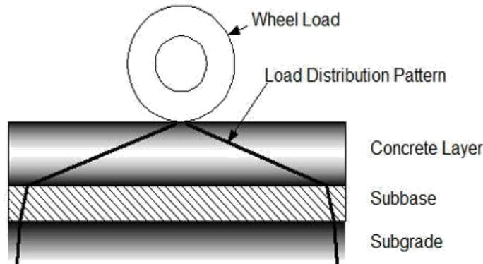
**Fig 2. Load distribution of rigid pavement.**
