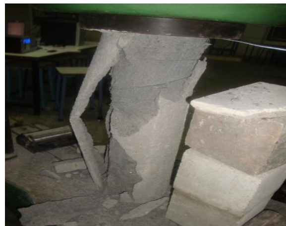
Fig. 3. Failure of confined specimens.
