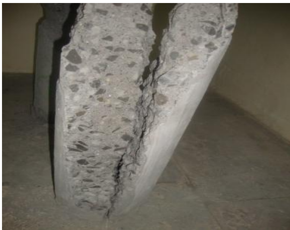
Fig. 2. Failure of unconfined specimens.
