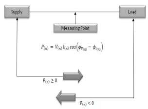
Fig. 1.0 Principle of locating nth harmonic source on the basis of its active power measurement.
