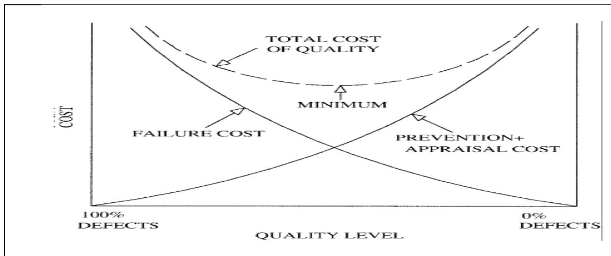
Fig.2. The basic model of optimum quality cost [6]
