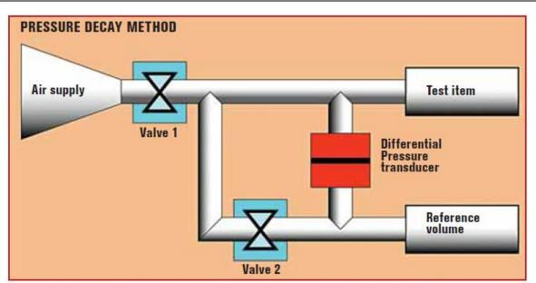
Test item and reference volume are pressurized and then isolated from the source by closing valve 1. Reference volume is then isolated from test item by closing valve 2, but they remain connected by a differential pressure transducer. Transducer reads pressure differential between non-leaking reference volume and leaking test item twice over a known time interval. The leak rate is calculated from the change in pressure, and the time over which it occurred.
