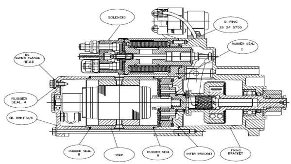
Fig. 1.1 Gear Reduction Starter Sectional view
