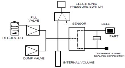
Fig 3.2 Sealed component measurement
