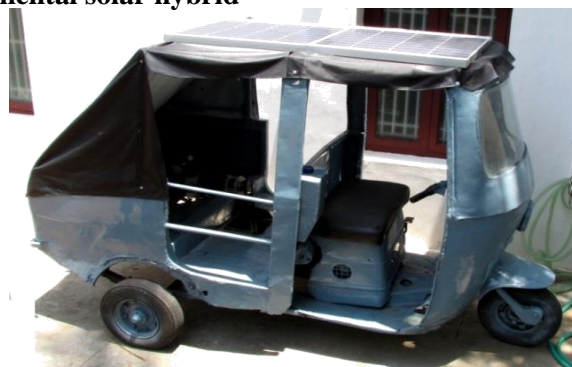
Fig. 4 solar hybrid auto rickshaw
