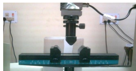
Figure 3.3 (b) Flexural specimen loading position
