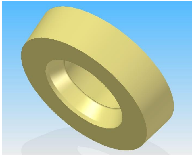
Figure 2. Model of Draw Die (seizing plate)
