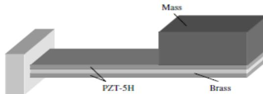
Fig. 4 Schematic of cantilever piezoelectric generator developed by Roundy [4]
