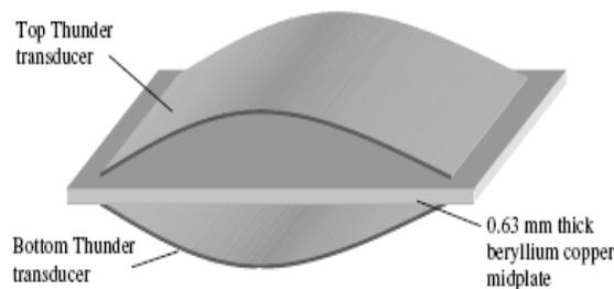
Fig. 3. Schematic of the piezoelectric dimorph (After Shenck)
