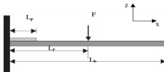
Fig. 5 Cantilever Beam with attached PZT sensor
