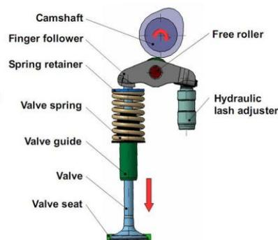
Fig.1. Engine valve mechanism
