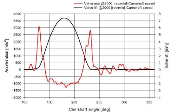
Fig.6. Valve acceleration versus Valve lift
