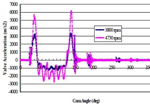
Fig.5. Valve acceleration comparison
