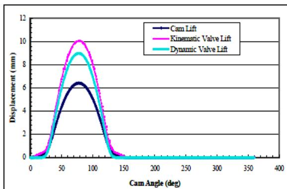
Fig.2. Displacement comparison [4]
