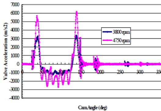
Fig.5. Valve acceleration comparison
