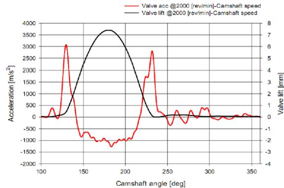
Fig.6. Valve acceleration versus Valve lift
