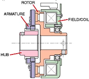
Fig 2: Electromagnetic clutch
