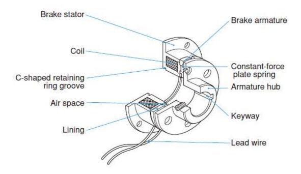
Fig 3: Electromagnetic brakes
