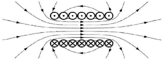
Fig 4: Magnetic Field Lines
