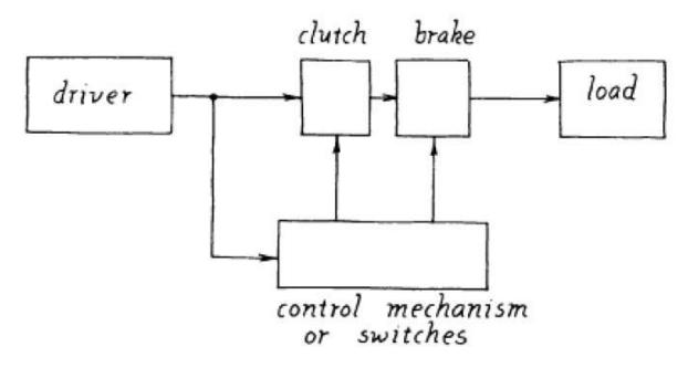
FIG.1 Construction of transmission system
