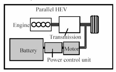
Figure 2: Schematic of a Parallel Hybrid Electric Vehicle [9]
