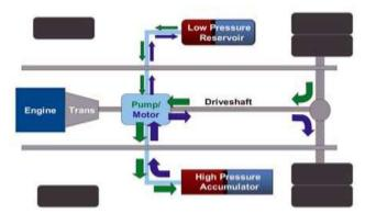
Figure 3: Schematic of Hydraulic RBS
