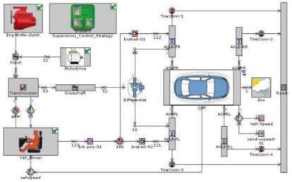
Figure 8. Parallel HEV planet model[8]
