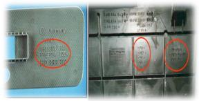
Fig.6. Material marking
