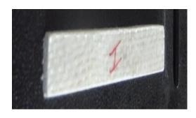
Length = 64mm, width = 12mm, thick = 5mm.
