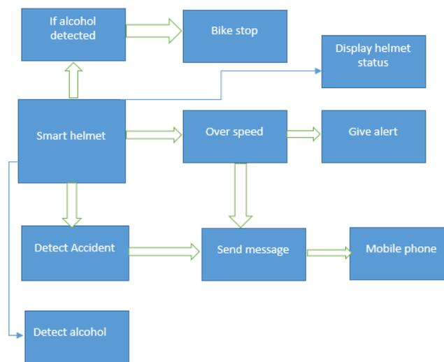
**Fig. 1.** Block diagram of Smart helmet
