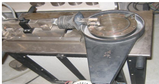
Fig. 1 Schematic view of the pin-on-disc apparatus used in this study.
