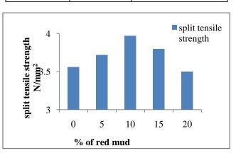
Figure 3. 28 Days split tensile strength without hydrated lime
