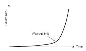
Fig. 1: Failure rate with identifiable wear out limit
