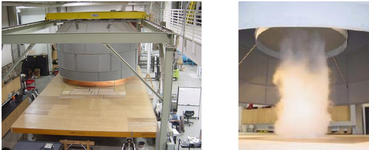
Fig.3 Photo of tornado simulator (circular duct) (designed in IOWA State University Wind Tunnel Lab) mounted on an overhead crane to move above the ground plane.
