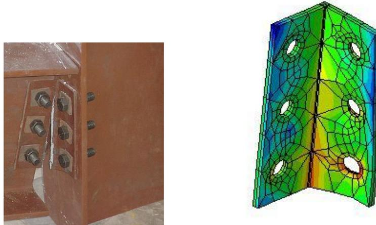
Fig. 5 Comparison of failure of the connection
