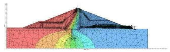
Figure 5: Flow network and seepage from dam Source: Kamanbedast and Delvari, 2012.
