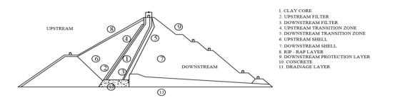
Figure 2: Cross Section of Ilam Dam After: Hasani, Mamizadeh and Karimi (2013)
