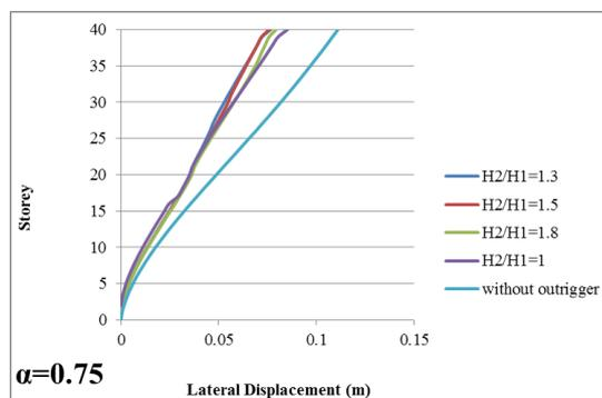
Figure 4: lateral displacement variation of multi-outrigger structure and core wall structure without outrigger for  $\alpha=0.5$  and  $\alpha=0.75$ .
