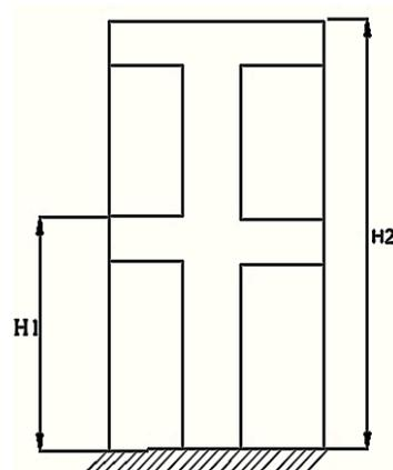
Figure 3:Relative height of outrigger
