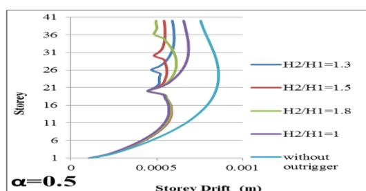
Figure 5: Storey drift variation of multi-outrigger structure and core wall structure without outrigger for  $\alpha=0.5$ .
