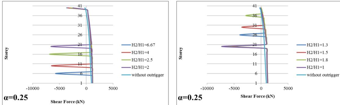
Figure 6: Shear force variation of multi-outrigger structure and core wall structure without outrigger for  $\alpha=0.25$ .
