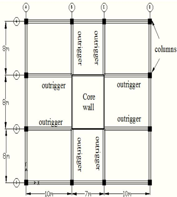
Figure 1: Plan of model considered
