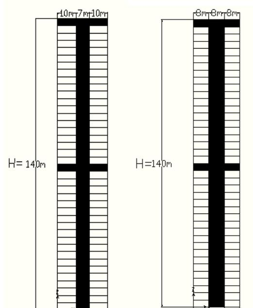
Figure 2: Elevation of model in X-Z and Y-Z direction
