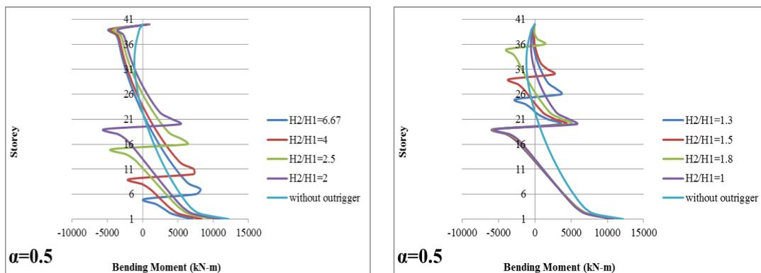
Figure 7: Bending moment of multi-outrigger structure and core wall structure without outrigger for  $\alpha=0.5$ .
