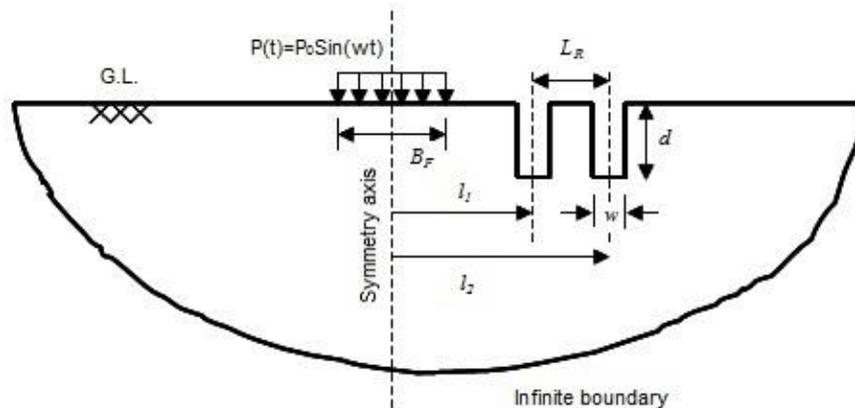
**Figure 1: 2-D schematic of the vibration isolation scheme on an elastic half-space**
