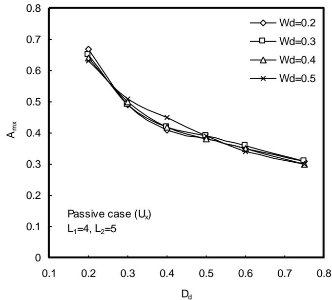
**Figure 5(b): Effect of depth and width of trenches on reducing horizontal vibration (passive case)**
