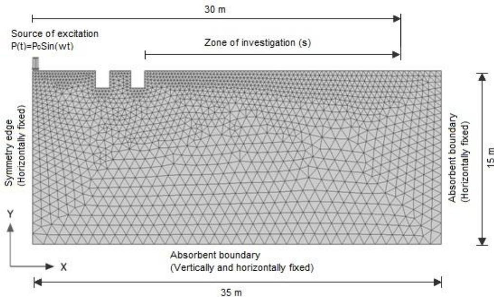
**Figure 2: A typical finite element model**
