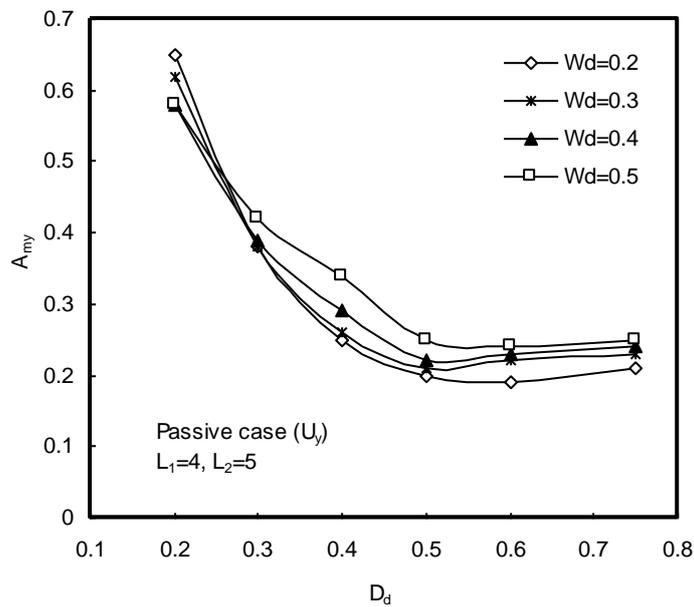
Figure 5(a): Effect of depth and width of trenches on reducing vertical vibration (passive case)
