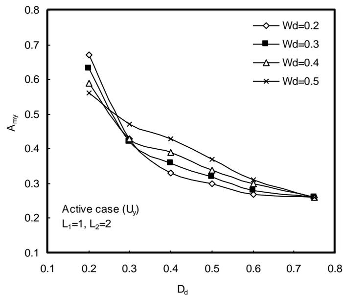
Figure 4(a): Effect of depth and width of trenches on reducing vertical vibration (active case)
