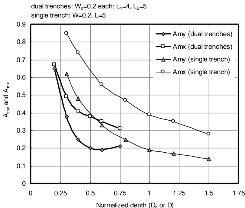
**Figure 6: Comparison of screening effectiveness of dual trench barrier over a single trench**
