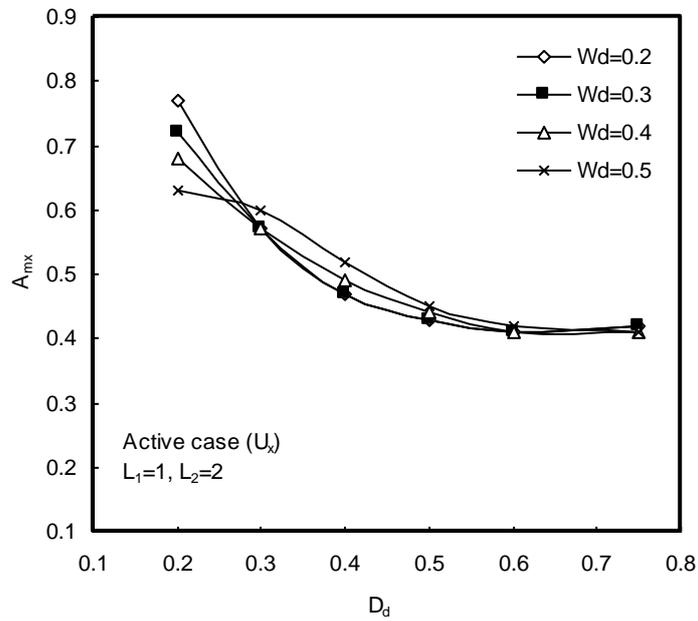
Figure 4(b): Effect of depth and width of trenches on reducing horizontal vibration (active case)
