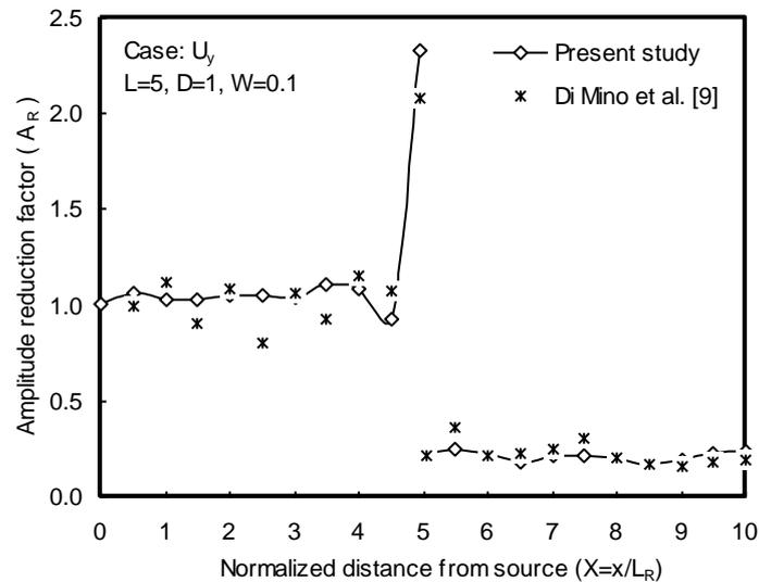
**Figure 7: Comparative study on vibration isolation by an open trench**
