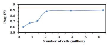
Fig.5: Grid independent study for bare hull
