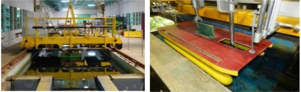
Fig.7: Experimental setup for drag test
