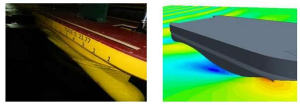
Fig.8: Flow pattern freeze shot around the hull from experiment and numerical simulation result from CFD. Flow kinematics are captured very well in the numerical model.
