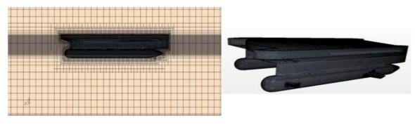
Fig.3: Volume mesh around the hull and at free surface
