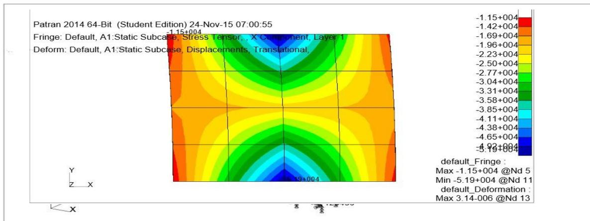
Fig.6 Finite element model of target plate modeled with human surrogate target as elastic support
