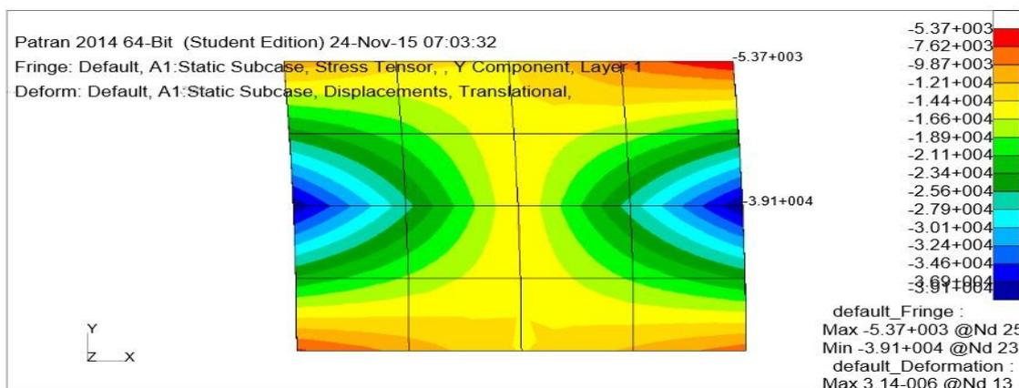
Fig.8 Longitudinal stress for layer 1 of curved laminated composite with human surrogate target
