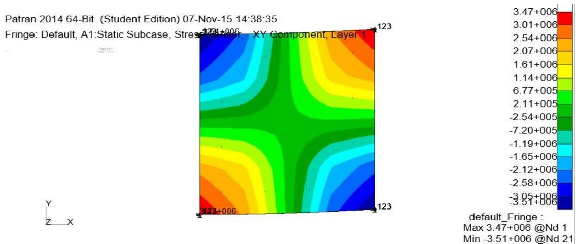
Fig.5 Shear stress for layer 1 of curved laminated composite
