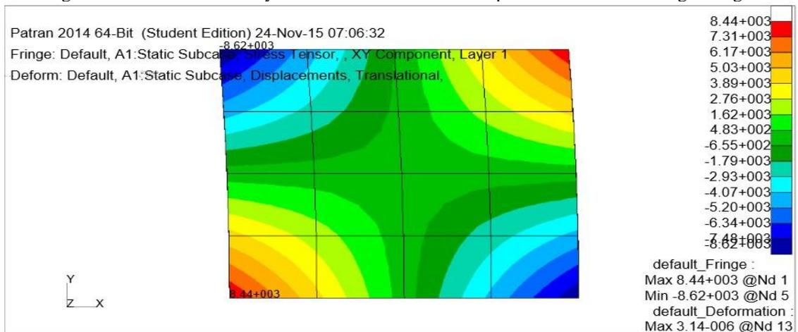
Fig.10 Shear stress for layer 1 of curved laminated composite with human surrogate target
