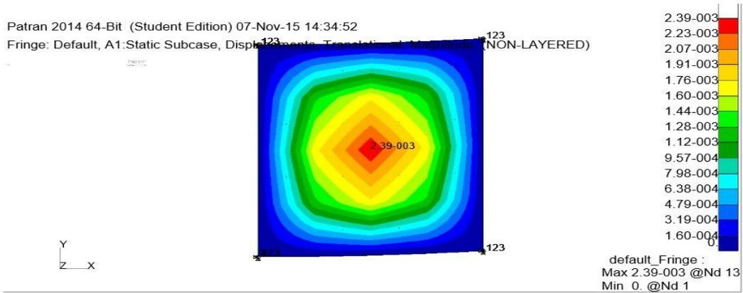
Fig.2 Deformation of curved laminated composite
