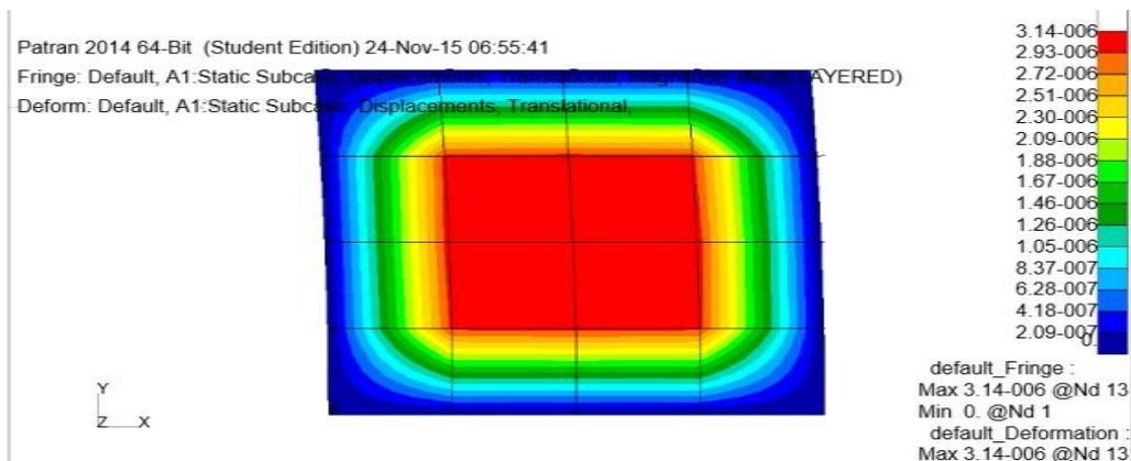
Fig.7 Deformation of curved laminated composite with human surrogate target
