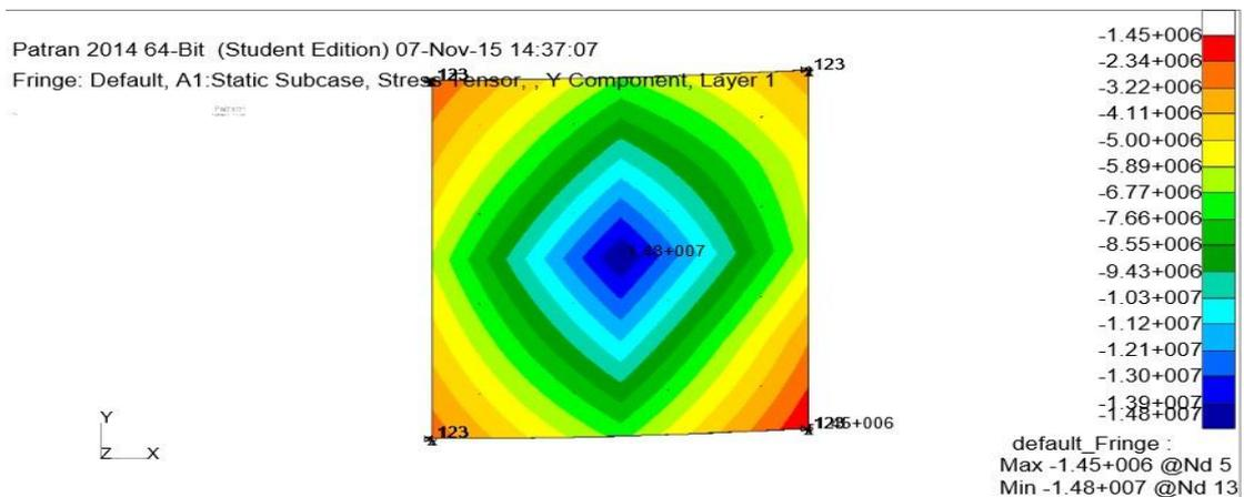
Fig.4 Transverse stress output for layer 1 of curved laminated composite
