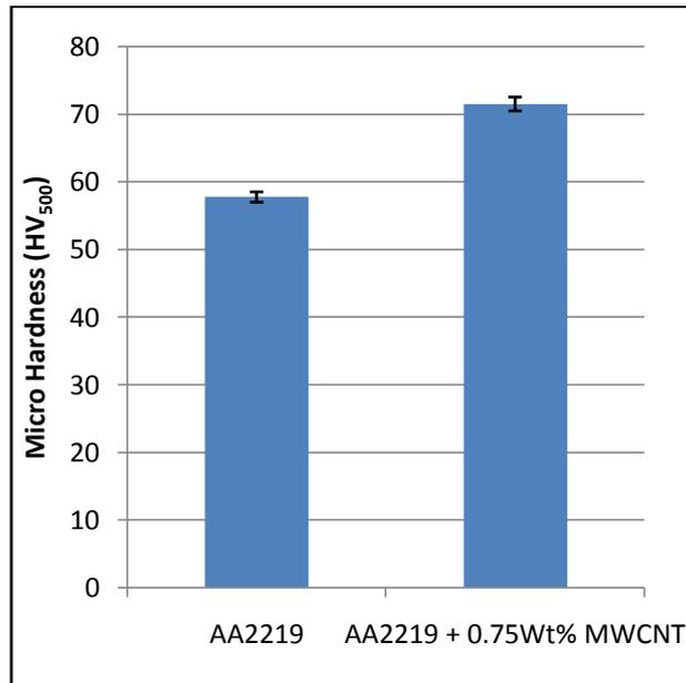
Fig 2: - micro hardness values for AA2219 and with 0.75wt% MWCNT addition.
