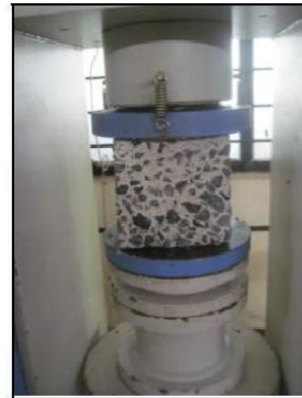
Fig 5: Compression test of concrete before acid attack Fig 6: Compression test of concrete after acid attack
