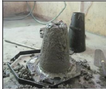
Fig 2: Slump check of concrete
