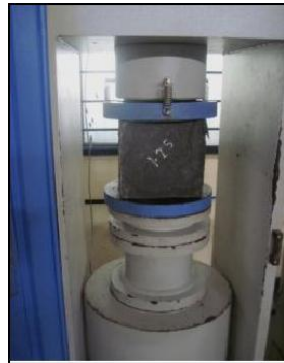
Fig 5: Compression test of concrete before acid attack Fig 6: Compression test of concrete after acid attack
