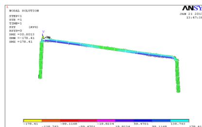
Fig: Maximum Shear Stress of 30 mm dia.
