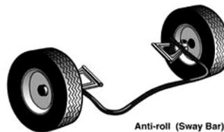
Figure 2.1 - A typical anti-roll bar
