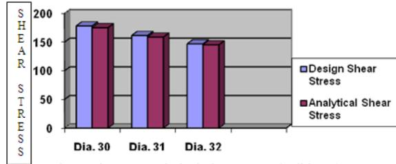
Fig: Design Vs Analytical Shear Stress (Solid Bar)
