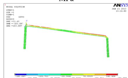
Fig: - Maximum Shear Stress of hollow bar
