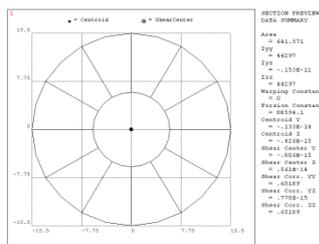
Fig: - Cross Section of Hollow Stability Bar
