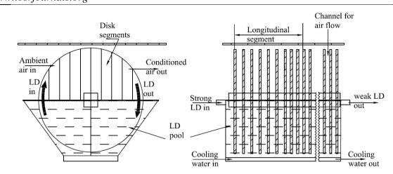
Fig. 3: Configuration and methodology of simulation for RDCD
