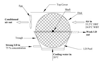
Fig. 2: Rotating disk type contacting device along with process parameters used in this work
