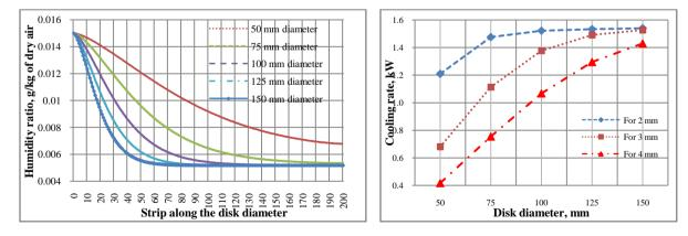
Fig. 4: Variation of humidity ratio of air along the diameter of the disk (depth of the channel)
