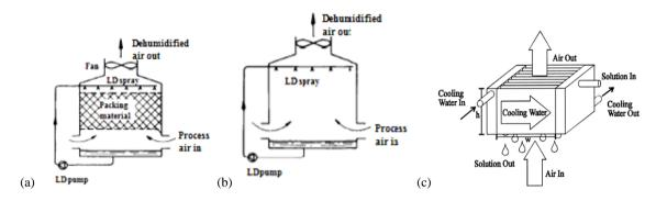
Fig. 1: Various types of LD-air contacting devices (a) Packed bed (b) Spray tower (c) Falling film
