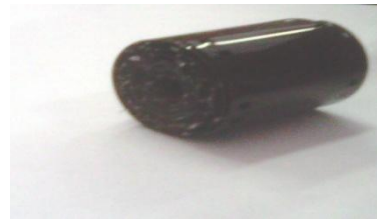
Fig.5 Stack used in thermo-acoustic refrigerator model
