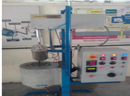
**Fig.1** Experimental setup used for stir casting.
