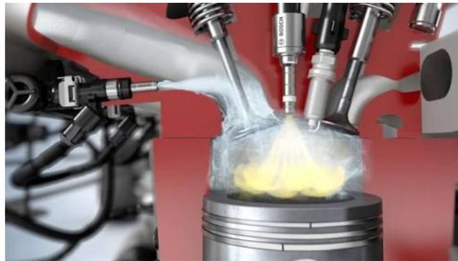
Fig. 2: In-Cylinder Type of Water Injection
