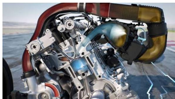
Fig. 3: Fumigation Type of Water Injection
