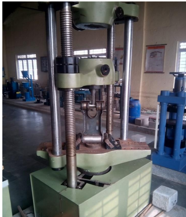
Fig.27: Compression testing on Universal Testing Machine
