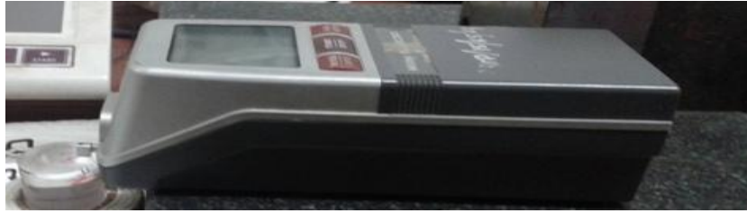
Fig.4 Surface roughness measurement using Talysurf
