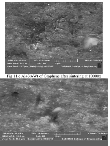
Fig 11.d Al+8% Wt of Graphene after sintering at 10000x
