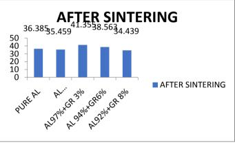
Fig.8 BHN value v/s wt.% of Graphene (After Sintering)
