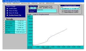
Fig 10a Load Vs Displacement for 1%.Wt of Graphene
