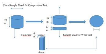
Fig. 9 Flow diagram of Preparation of Samples for Wear Test
