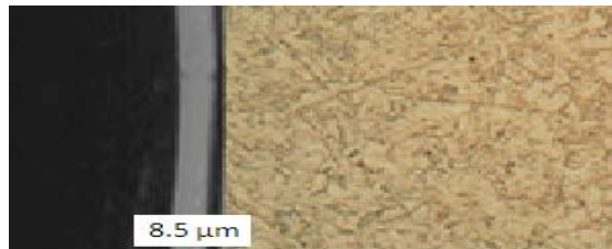
Fig 3: Flame Hardening for 1 min
