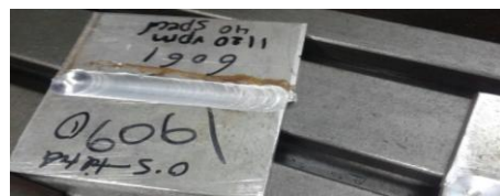
Fig 4 Sample 3 6061-6061 With Taper Tool
