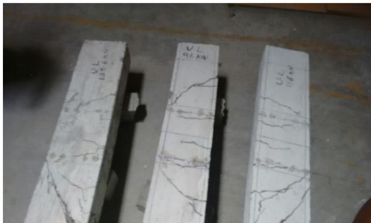
Fig 9 Crack pattern in beams
