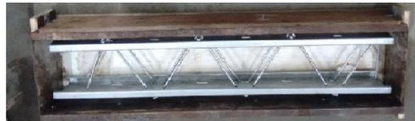
Fig.3 Laced Reinforced Beam
