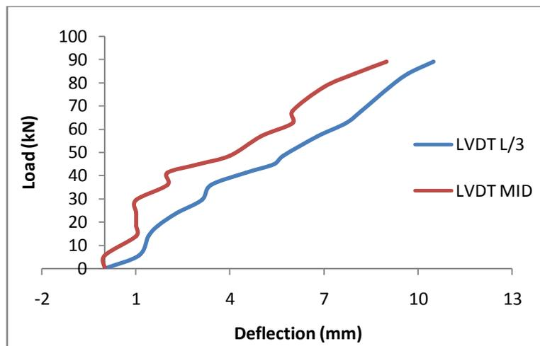
Fig 7 RC Load vs Deflection
