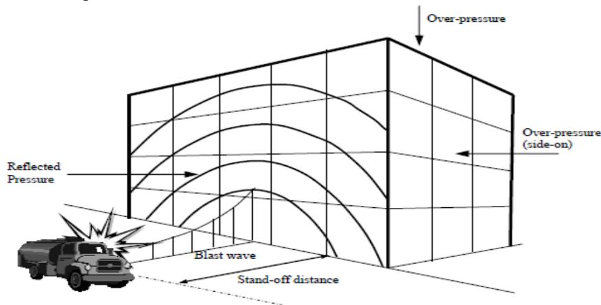
Fig.1 Blast Load effect on Building
