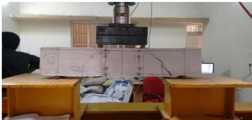
Fig.4 Experimental setup of Beam in Loading Frame
