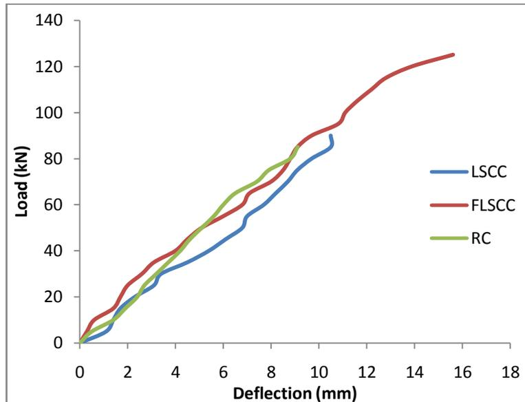
Fig 8 Comparison of LSCC, FLSCC and RC
