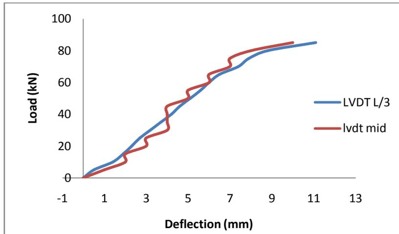
Fig 6 FLSCC Load vs Deflection
