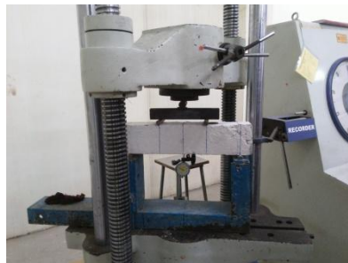
Fig 6 Flexural strength testing of beams
