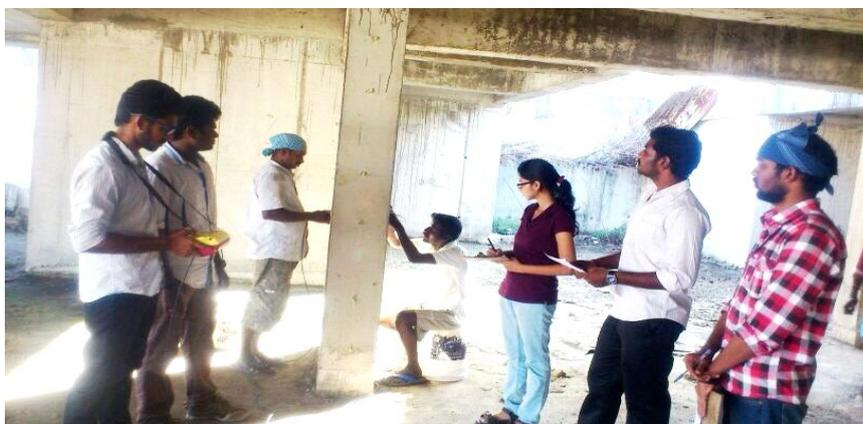
Fig. 2 Ultra-Sonic Pulse velocity Test
