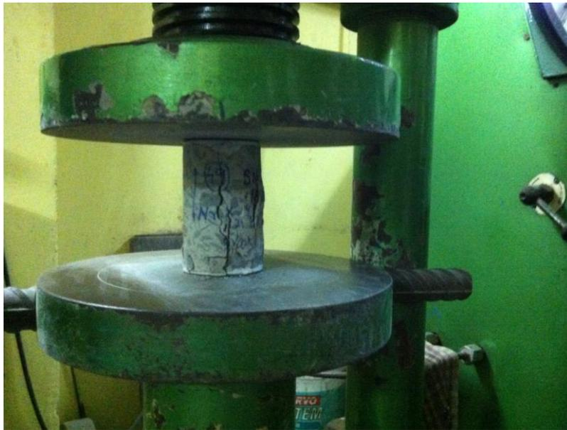
Fig 3 Core Sampling Test
