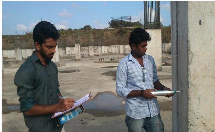
Fig .1 Rebound Hammer Test
