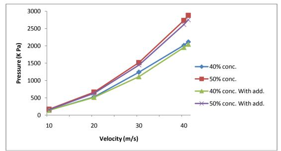
Fig.3. Pressure Drop per 100 meter Length with Different Flow Velocity and % Concentration for Water and Bottom Ash Mixture with 2% Additive in Straight Pipe
