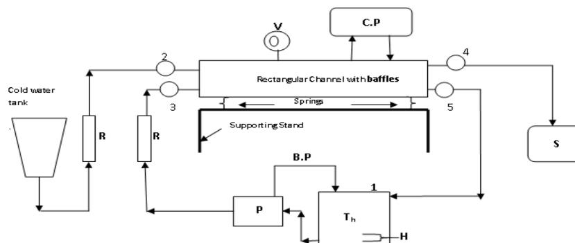
Fig. 1 Schematic diagram of rectangular heat exchanger with vibrator
