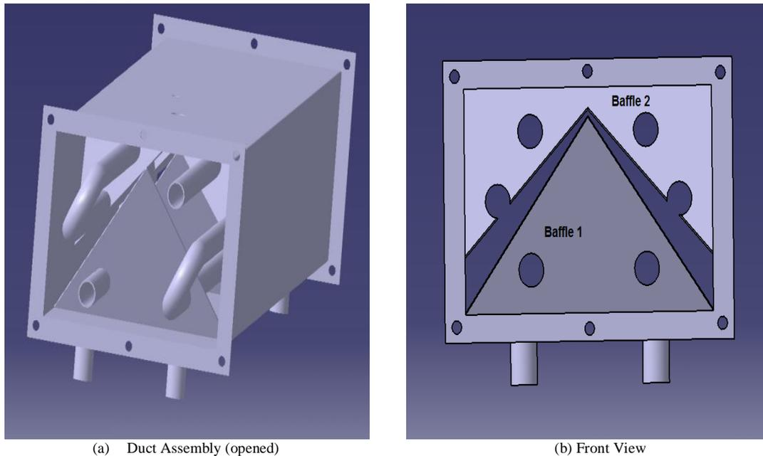
Fig. 2 Different views of rectangular channel.
