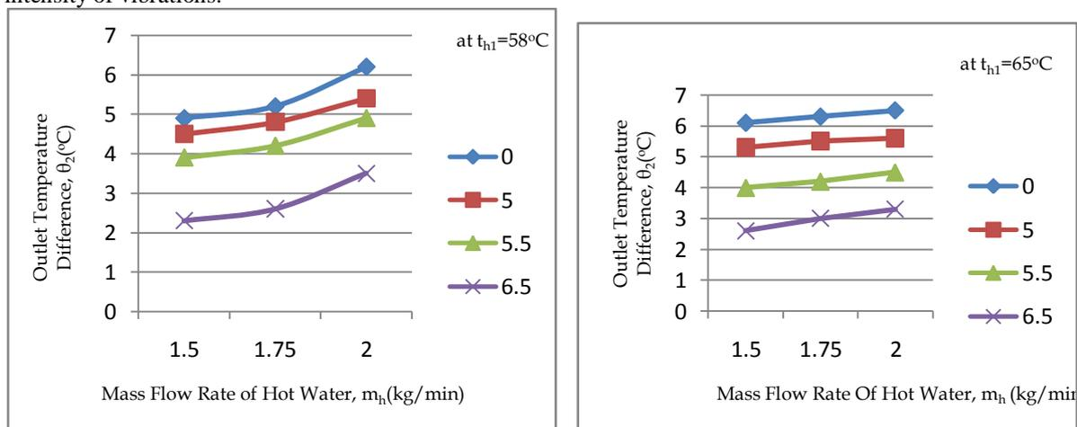
Fig. 3.2 Effects of vibrations on outlet temperature difference at different mass flow rate of hot water (at  $t_{hi} = 58^\circ\text{C}$  &  $65^\circ\text{C}$ )
