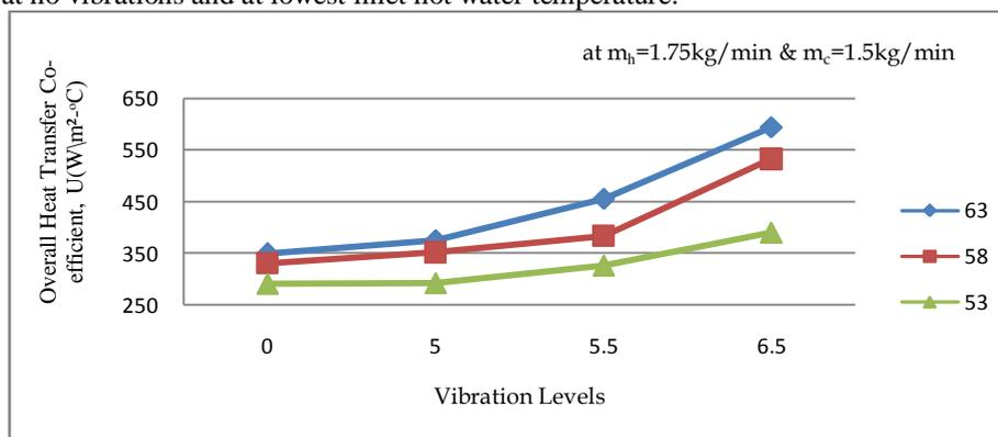
Fig. 3.4 Variation of overall heat transfer co-efficient with vibration levels at different hot water inlet.
