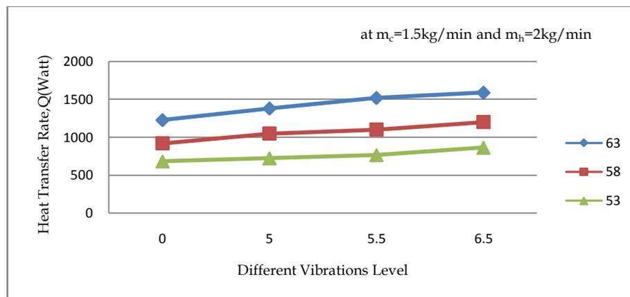
Fig. 3.3 Effect of heat transfer rate of hot water with vibration levels at different inlet hot water temperature.
