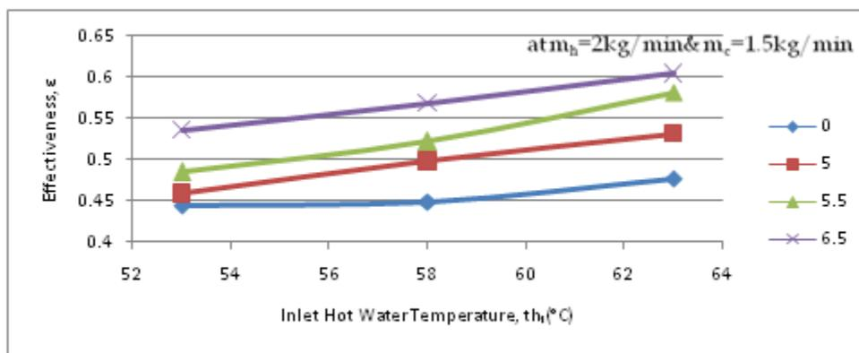
Fig. 3.5 Effect of inlet hot water temperature on effectiveness at different vibration levels
