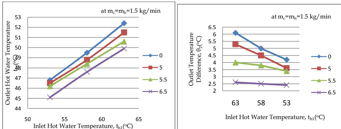
Fig. 3.1 Effects of outlet hot water temperature and outlet hot water difference with inlet hot water temperature at different vibration levels
