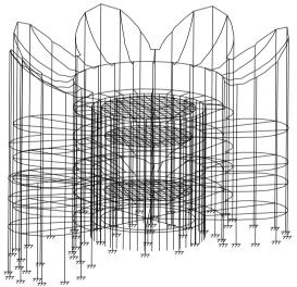
Fig.8. Structural model of media exhibit building
