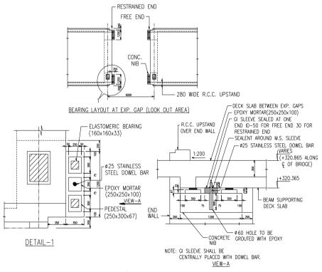
Fig.4. Support arrangement for intermediate slab between two arch bridges
