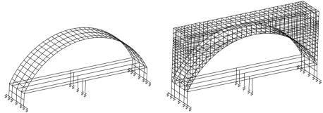
Fig.7. Construction stage and service stage models for the arch bridge
