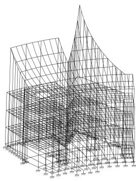
Fig.9. Structural model of part of permanent exhibit building
