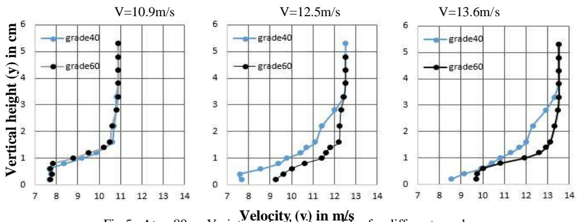
Fig.5. At x=80cm Variation of velocity profiles for different roughness
