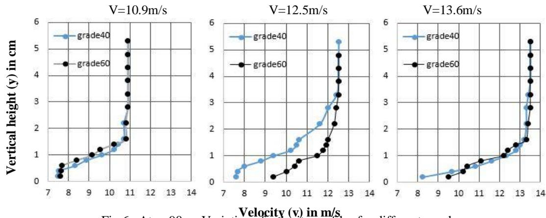
Fig.6. At  $x=90\text{cm}$  Variation of velocity profiles for different roughness
