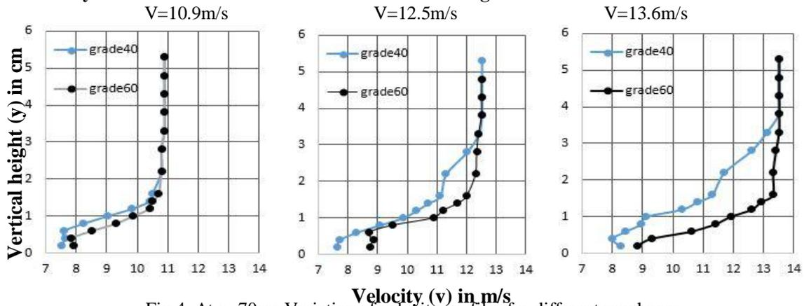
Fig.4. At x=70cm Variation of velocity profiles for different roughness
