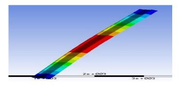
Fig 6 Column deformed under blast pressure.
