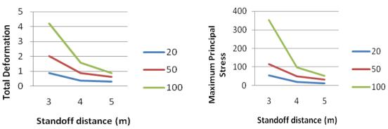
Fig. 7 Stand-off distance Vs Deformation
