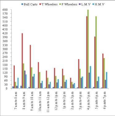
Fig.4. Traffic Volume Banur to Landran (Peak Hour 9-10am, 5-6pm
