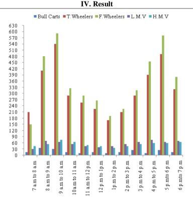
Fig.2. Traffic Volume Landran to Chandigarh (Peak Hour 9-10am, 5-6pm)
