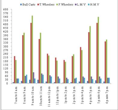
Fig.3. Traffic Volume Chandigarh to Landran (Peak Hour 9-10am, 5-6pm)
