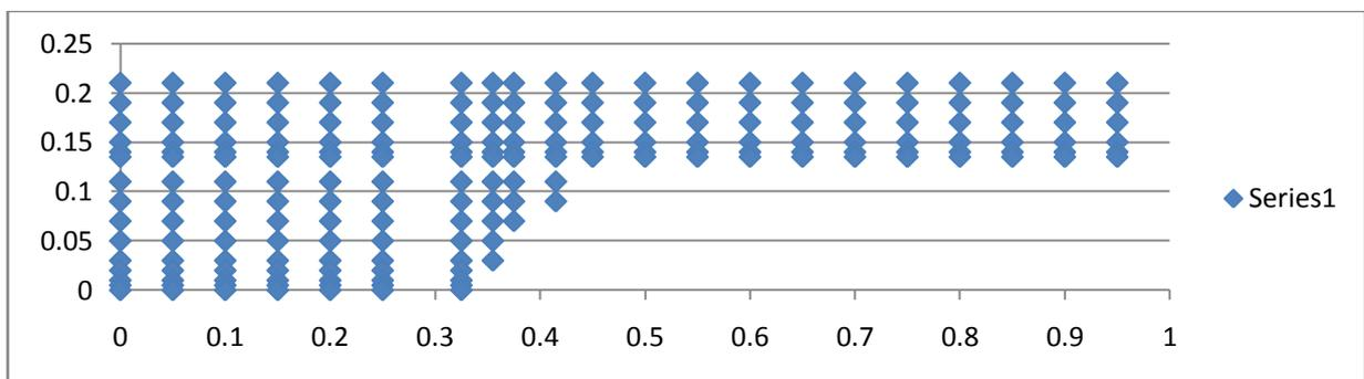
Fig 2.5: TYPICAL GRID POINTS FOR MEASUREMENT OF VELOCITY
