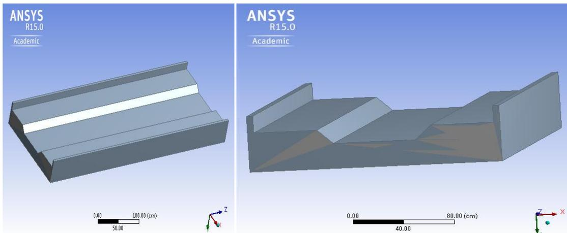
**Fig 2.6: GEOMETRY OF COMPOUND CHANNEL WITH ROUGH FLOOD PLAIN**
