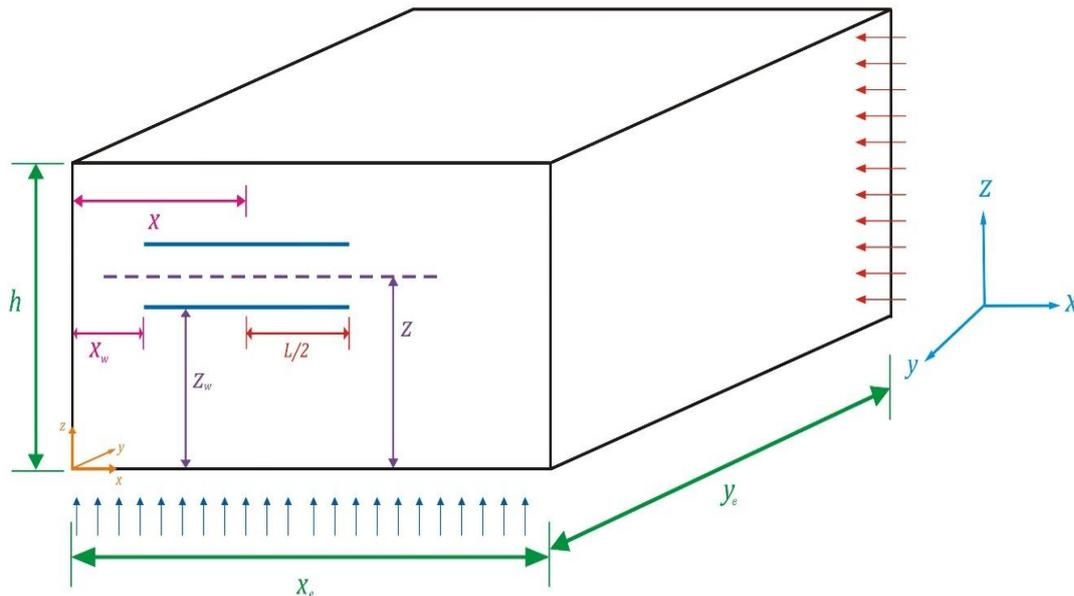
Figure 1: Horizontal well acting in an infinite reservoir
